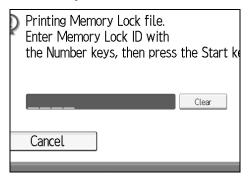
If the Memory Lock ID does not match, the "Specified code does not correspond to programmed Memory Lock ID." message appears. Press **[Exit]** and retry after checking the Memory Lock ID.
